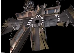
(c) Outdoor point cloud delivered by the LiDAR Leica P20 with 72 947 044 points
