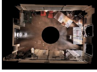
(b) Indoor point cloud after sampling containing 986 344 points
